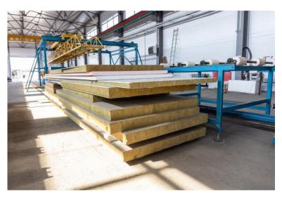
required, like in Pre-engineered buildings, warehouses and cold-chain solutions. PU panel has low thermal conductivity (R-value). R-value is an important measure of resistance to heat flow through a given thickness of material. R-value figures of PU panels are given in the table (The lower the better).
